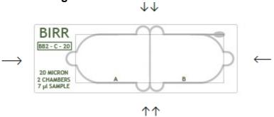
Two chambers, A and B.  $\rightarrow$  Point to filling place of chamber A;  $\leftarrow$  point to filling place of chamber B.  $\uparrow \uparrow$ ,  $\downarrow \downarrow$  air outlets
